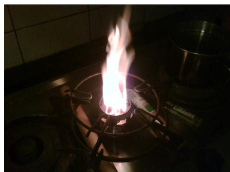
*Canted holes in the Twister Lite give its flames a cyclonic action. The added internal flute construction helps to direct the flame plasma in a cyclonic pattern. The flutes act as directional baffles.*
