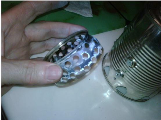
I cut off the top portion of a steel Coca Cola tin and then punched it full holes with a paper punch and a lot of grunting and squeezing. Steel tins are so much tougher than aluminium!
