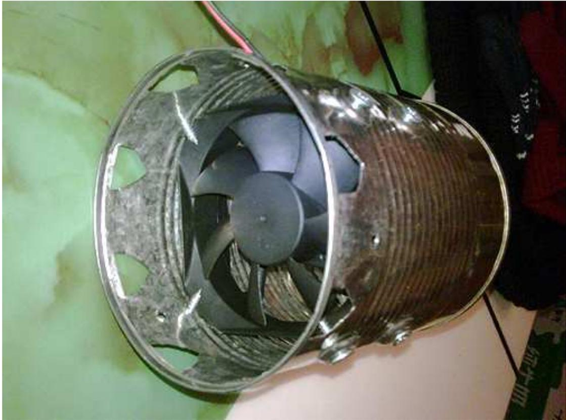
*Computer 4" fan mounted by breaking off corner tabs and slipping it into the tin.*
