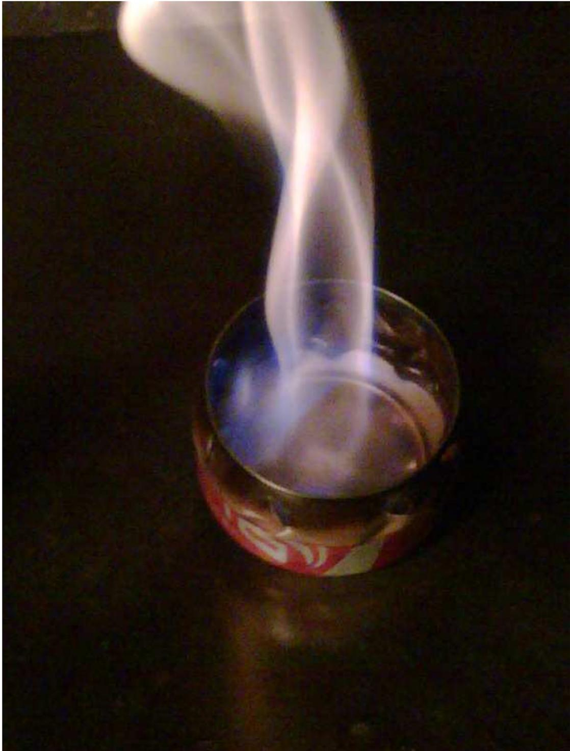
*A thing of beauty is the Twister Lite in passive mode. Canted air intakes provide a cyclonic action which is aided by the flutes inside the chamber. I am not sure how much help the flutes provide but "it couldn't hurt".*
