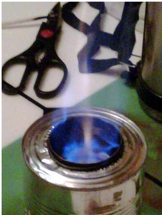
*I used a fruit tin, cut a hole in the bottom and inserted Twister Lite from within.*
