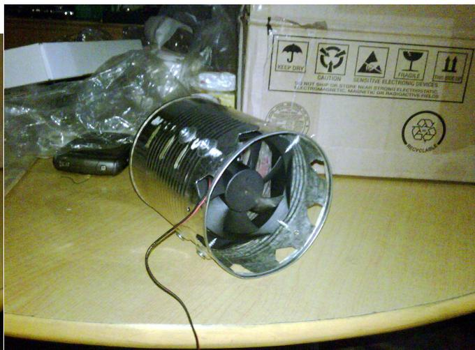
The fan is mounted a couple inches below the cooker bottom and just above the air intake holes. The distance from the cooker protects it from the heat and the distance above the air intake holes assures unimpeded air intake. I cut the corner tabs off the fan with a pair of diagonal cutting pliers in order to snug it up into the tin.
