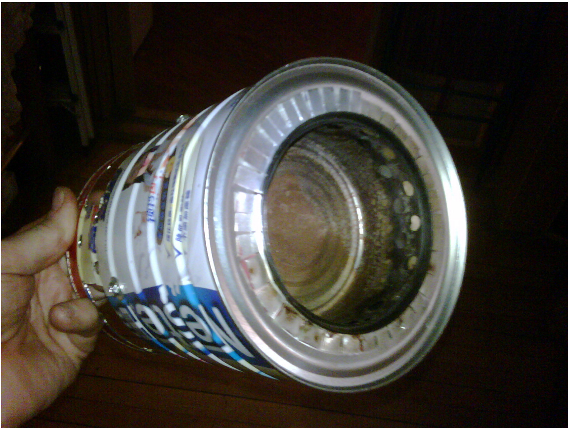
I inserted my CAT (Turbo Tuna Surprise) in the hole. The fringe you see is aluminium stripping from a soda tin I used to fill a slightly oversized hole.
