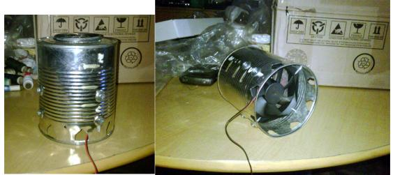
The fan is mounted a couple inches below the cooker bottom and just above the air intake holes. The distance from the cooker protects it from the heat and the distance above the air intake holes assures unimpeded air intake. I cut the corner tabs off the fan with a pair of diagonal cutting pliers in order to snug it up into the tin.
