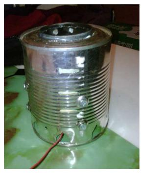
The tin is inverted with the bottom now the top. Twister Lite can be seen sticking his head out, supported by the snap ring. At the bottom are air inlet holes cut in with a church key can opener. The wires protruding through an airhole are for the electricity to power the electric 4" computer fan mounted inside. It works.
