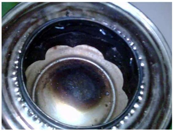
Twister Lite held up by a "snap ring" made from a coat hanger.
