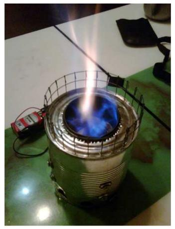
On 95% alcohol and both batteries she burns HOT! This is good for a 90 second boil time and does the job very quickly. Makes a soft turbo sound too. The fan is quiet, but the flame is not.
