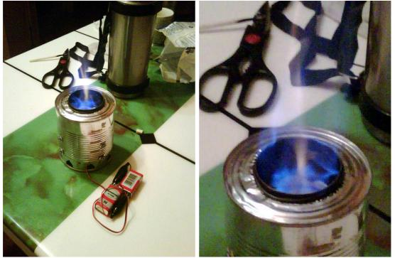
I used a fruit tin, cut a hole in the bottom and inserted Twister Lite from within.
