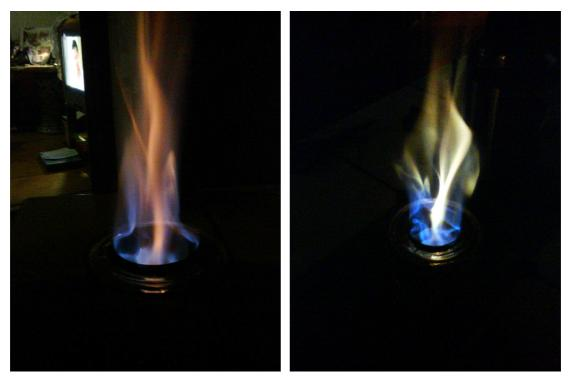
El Diablo blowing a blue streak on 95% isopropyl alcohol. "Up, up, and away." 9V on the left, 18V on the right. The fan is rated  $9 \sim 24V$
