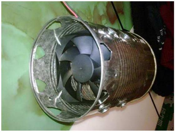
Computer 4" fan mounted by breaking off corner tabs and slipping it into the tin.
