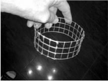
Take a close look and you'll see that the "round-pod" has been fitted exactly to the top of El Diablo. This actually sits barely within the raised rim of the tin providing a secure seat for the pot and a reinforced strength by utilizing the lip on El Diablo.
